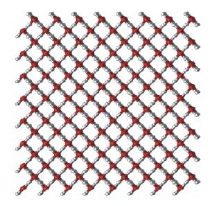
The melting curve for ice-ten has been proposed at high temperatures (1000-2400 K) [612a]. As ice X is approached with increasing pressure from very hot liquid water and the O-H energy minima draw near to each other, the protons rapidly swap positions giving many short-lived  $OH^-$  and  $H_3O^+$  ions [612b]. In the ice X, however, protons are less mobile than in ice VII as there is only one energy minimum for each O-H-O bond,
