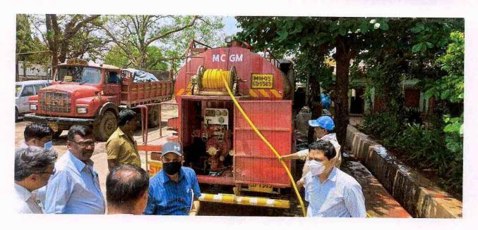
FIREX Water tankers (Fire Engine cum Water Tanker) of 10000 Liters Capacity each along with Sprinkler System
