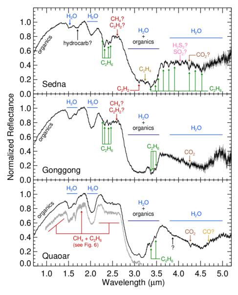
**Figure 2.** JWST NIRSpec spectra of Sedna, Gonggong, and Quaoar. All spectra are normalized to the mean between 1.8 and 1.9  $\mu$ m. The three dwarf planets share many spectral similarities, but they also differ in several interesting and important ways. The higher spectral resolution medium grating spectrum (shown in gray) of Quaoar resolves features not detected in the prism spectrum, but otherwise agrees very
